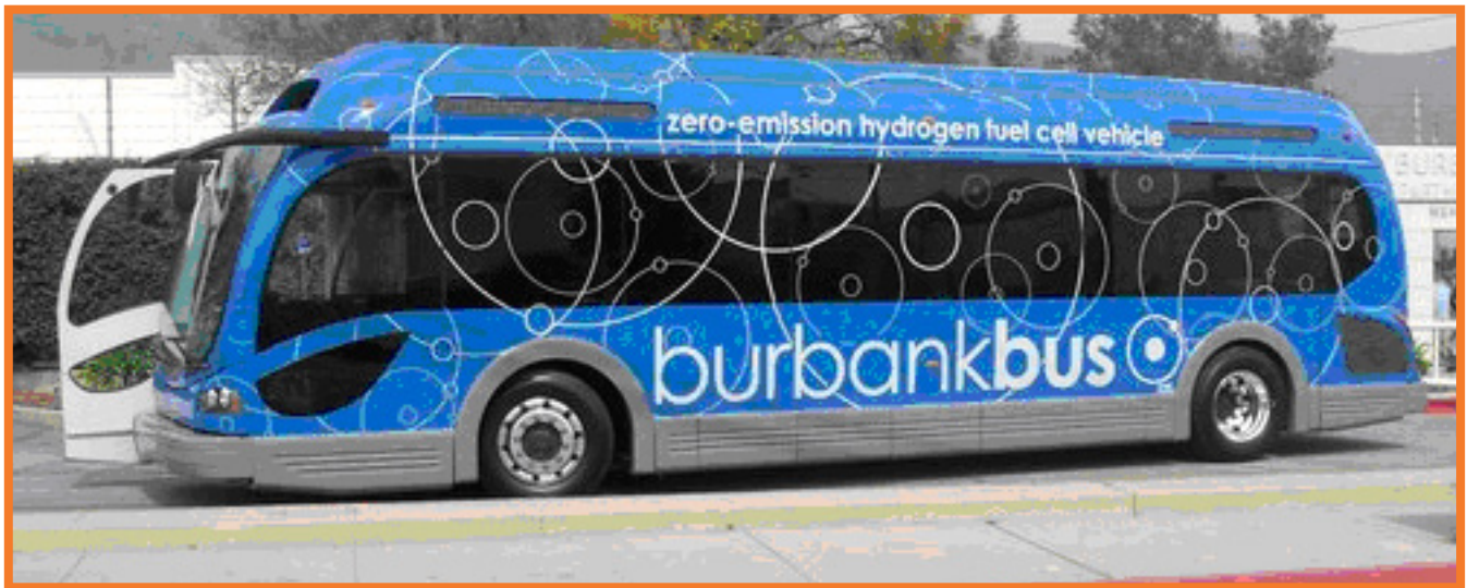
Hydrogen fuel cell bus. Source: National Renewable Energy Laboratory (NREL) Photographic Information eXchange (PIX) #17239
