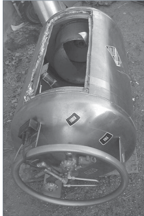
Figure 76: Cutaway of LNG tank showing dual walls and insulation. Source: NAFTC.
