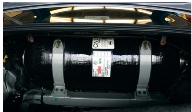
Figure 74: Photo of Type 4 cylinder. Source: NAFTC.
