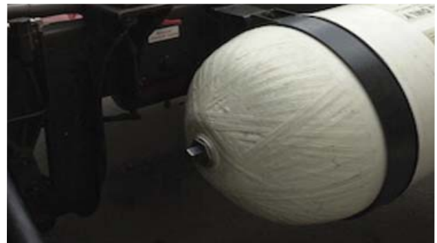
Figure 73: Photo of Type 3 cylinder. Source: NAFTC.
