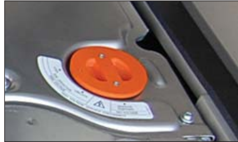
Figure 88: Hybrid high-voltage system disconnect. Source: NAFTC.
