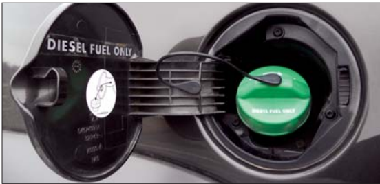
Figure 45: Diesel gas cap. Source: NAFTC.
