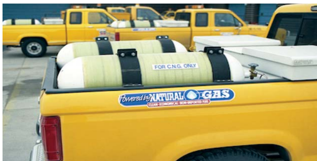
Figure 11: Photo of Type 2 cylinder. Source: NAFTC.
