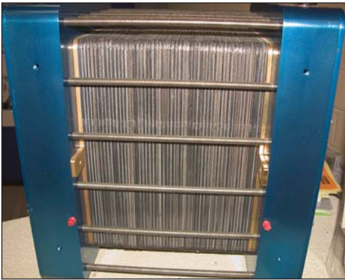
Figure 35: Cutaway view of a fuel cell. Source: NAFTC.
