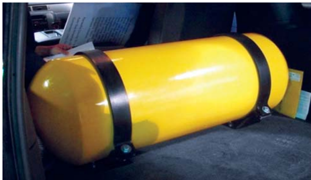
Figure 10: Photo of Type 1 cylinder. Source: NAFTC.
