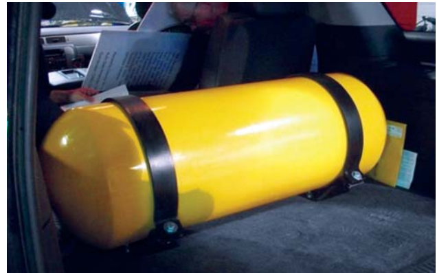
Figure 71: Photo of Type 1 cylinder. Source: NAFTC.
