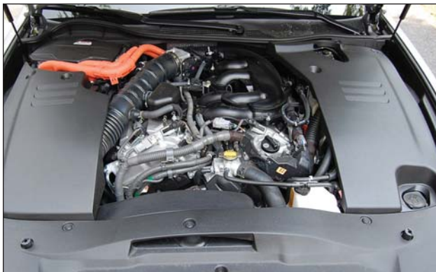
Figure 67: High-voltage cables under the hood of a hybrid electric vehicle. Source: NAFTC.
