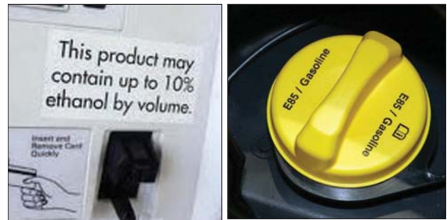
Figure 47: Fuel pump label for ethanol. Source: NAFTC. Figure 48: E85 cap on a flexible fuel vehicle. Source: NAFTC.
