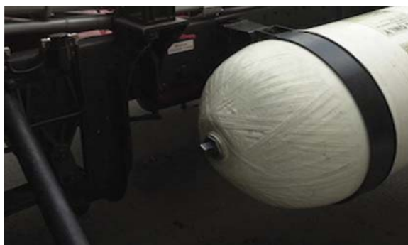
Figure 12: Photo of Type 3 cylinder. Source: NAFTC.
