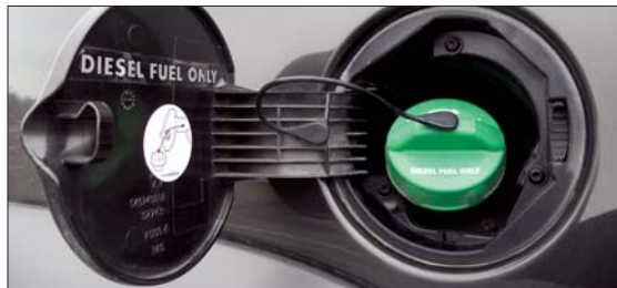
Figure 4: Diesel gas cap. Source: NAFTC.
