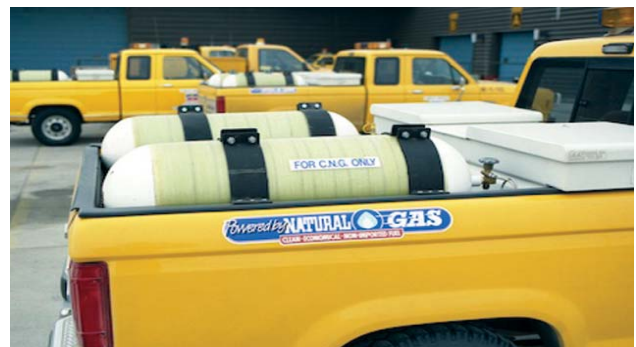
Figure 72: Photo of Type 2, steel-lined cylinder. Source: NAFTC.
