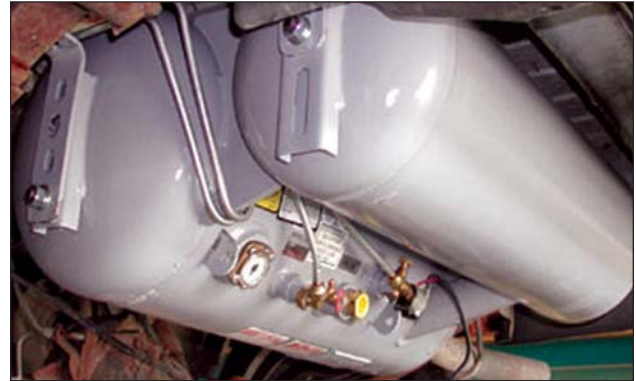
Figure 78: Propane cylinder with information on body. Source: AFDC.
