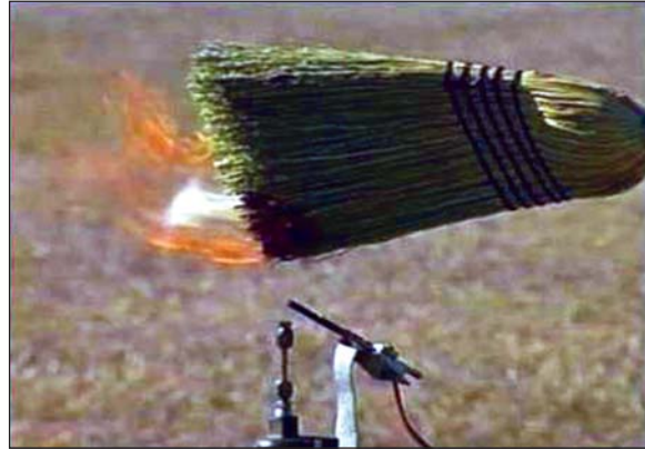
Figure 82: Hydrogen flame detected by broom. Source: AFDC.
