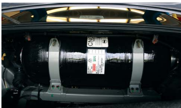
Figure 13: Photo of Type 4 cylinder. Source: NAFTC.
