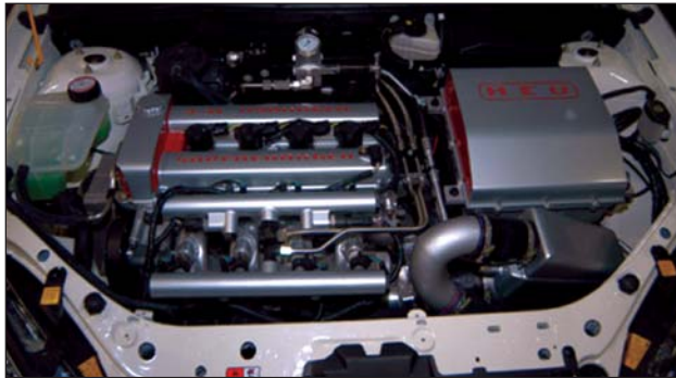
Figure 79: Hydrogen internal combustion engine compartment. Source: NAFTC.
