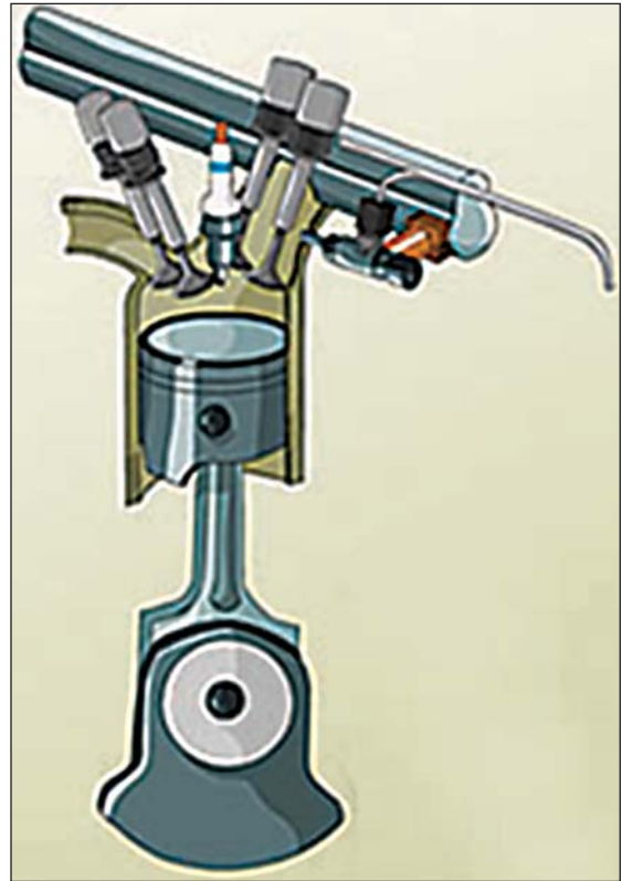
Figure 34: Hydrogen internal combustion engine components. Source: NAFTC.
