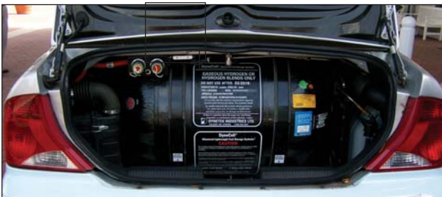
Figure 85: Location of hydrogen tank PRD vent. Source: NAFTC.
