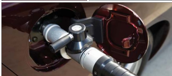
Hydrogen fueling port
