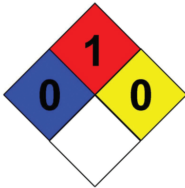
Figure 4: NFPA 704 hazard placard for B100 biodiesel. Source: NFPA.
