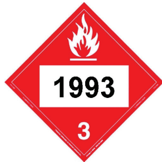
Figure 5: Hazardous material description identifies number UN 1993 placard for diesel. Source: DOT, PHMSA.
