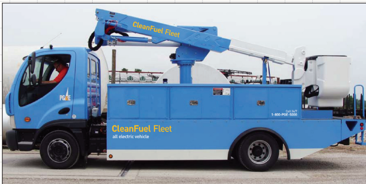
The PG&E 100% electric bucket truck, configured and manufactured by Smith Electric Vehicles. Photo courtesy of PG&E.
