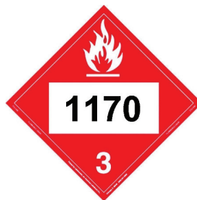
Figure 8: Hazardous material description identification number UN 1170 for ethanol. Source: DOT, PHMSA.
