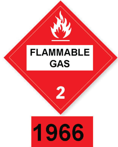
Figure 6: Hazardous material description identification number UN 1966 for liquid hydrogen. Source: DOT, PHMSA.
