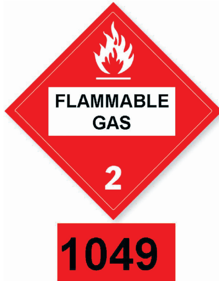
Figure 5: Hazardous material description identification number UN 1049 placard for gaseous hydrogen. Source: DOT, PHMSA.
