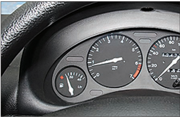
Tachometer indicating an idling engine. Source: NAFTC.
