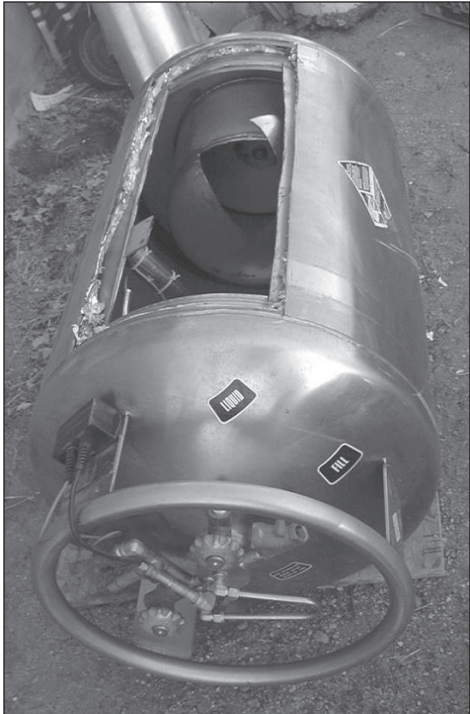
Figure 3: Cutaway of LNG tank showing dual walls and insulation. Source: NAFTC.
