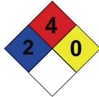
Figure 9: NFPA 704 hazard placard for LNG. Source: NFPA.
