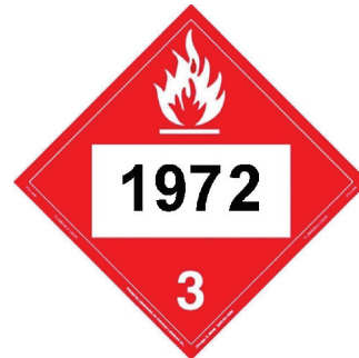
Figure 11: LNG transport placard UN 1972. Source: DOT.
