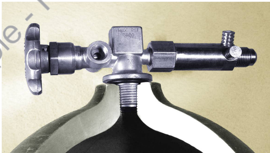
Figure 2-7: Manually-operated CNG cylinder valve, in cut-away Type 2 cylinder with pressure valve (PRD). SAE threads and O-ring shown. Photo Courtesy of NAFTC.
